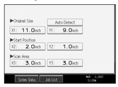
Specify Start Position (X2 and Y2) using the number keys, and then press the [#] key.
